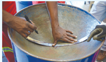
Instructor demonstrating marking the pan for notes
