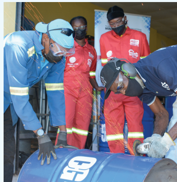
Instructor demonstrating smoothing of the drum
