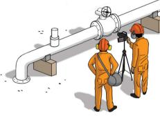
NGC integrated satellite data and an infrared camera to visualise leaks along its infrastructure, to improve asset integrity and risk management and support methane emissions reduction.
